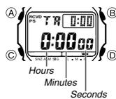
You can set the countdown timer within a range of one minute to 24 hours. An alarm sounds when the countdown reaches zero.
