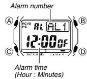
The Alarm Mode gives you a choice of four one-time alarms and one snooze alarm. Also use the Alarm Mode to turn the Hourly Time Signal (**SIG**) on and off.
