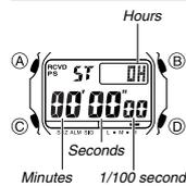
The stopwatch lets you measure elapsed time, split times, and two finishes.
