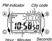
1. In the Timekeeping Mode, hold down (A) until the city code starts to flash, which indicates the setting screen.
