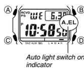
This watch has an EL (electro-luminescent) panel that causes the entire display to glow for easy reading in the dark. The watch's auto light switch turns on illumination automatically when you angle the watch towards your face.
