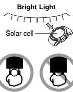
The electricity generated by the solar cell of the watch is stored by a rechargeable battery. Leaving or using the watch where it is not exposed to light causes the battery to run down. Make sure the watch is exposed to light as much as possible.
