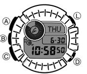
The display of the watch is illuminated for easy reading in the dark. The watch's auto light switch turns on illumination automatically when you angle the watch towards your face.
