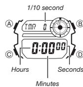
The countdown timer can be set within a range of one second to 24 hours. An alarm sounds when the countdown reaches zero.
