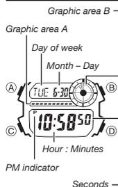
The Timekeeping Mode's Multi Time feature gives you quick and easy access to the current time and date in four different cities, numbered from T-1 (Time 1) through T-4 (Time 4). T-1 is your Home City Time, and T-2, T-3, and T-4 are Local Times. Local Times are kept in synchronization with your Home City Time (T-1).
