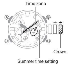
2. Hold down (C) for at least one second. This causes the second hand to move to 12 o'clock, and enables the minute setting operation.
