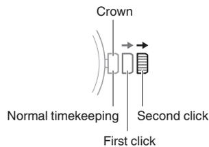
After pulling out the crown to the first or second click, rotating it quickly in succession in either direction will start a fast forward or fast reverse operation. While a fast forward operation is in progress, quickly rotating the crown in succession again will increase the speed even further.
