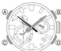
3. Within 10 seconds after you perform the operation in step 2, loosen the crown and then pull it out to the first click.
