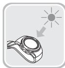
While you are wearing the watch, make sure that its face (solar panel) is not blocked from light by the sleeve of your clothing. Power generation efficiency is reduced even when the face of the watch is blocked only partially.
