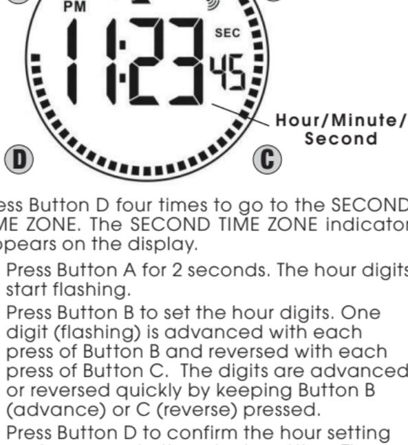
Press Button D four times to go to the SECOND TIME ZONE. The SECOND TIME ZONE indicator appears on the display.
